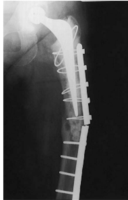
Fig. 1. Anteroposterior radiograph showing the failure of the periprosthetic femoral fracture fixation methods. Dall-Miles plate fracture from Tsiridis et al. (2003) with permission from Elsevier.
